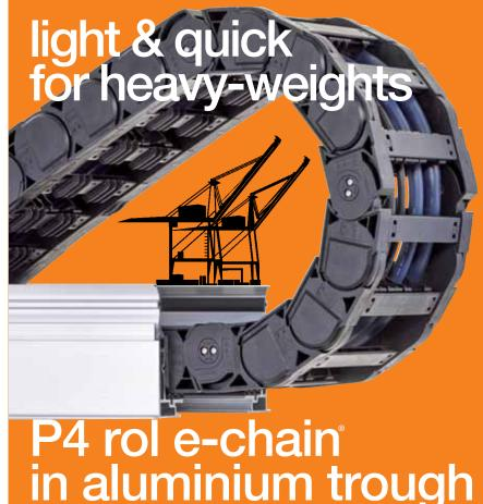
All media in a single e-chain. Drive and data cables, hoses, accessories. Corrosion-free and resistant to salt water in the igus<sup>®</sup> aluminium trough. Saves 30% weight compared to steel troughs. Travel of up to 800 m and speed of up to 600 m/min with 57% less drive power. Moving energy made easy.
